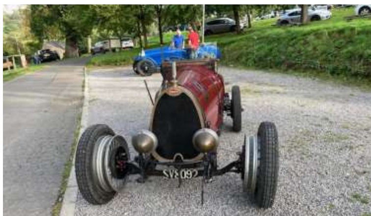
Rupert Marks used his Bugatti and put the twin wheels on the front instead of the rear to widen the track !
